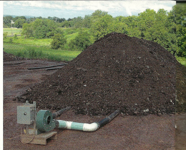
Temperature in an O2 Compost ASP System is regulated by adjusting the airflow coming into the pile.
