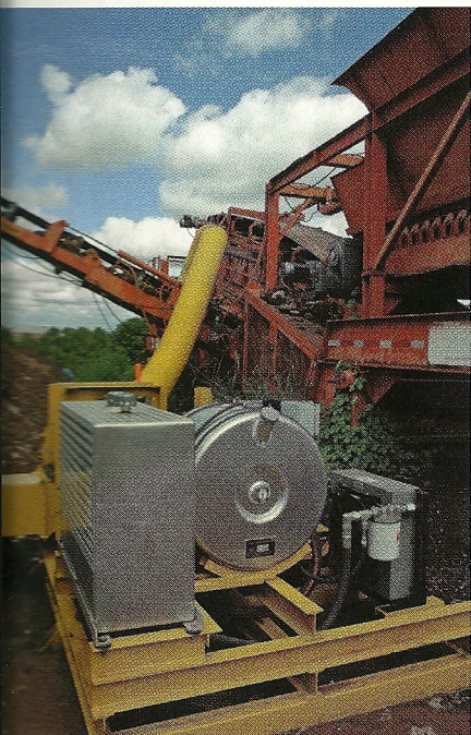
An Airlift separator helps remove plastic and other lightweight materials from the compost.
